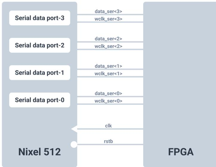
The Nixel 512 chip has five digital inputs and twelve digital outputs (I/Os) connected to the world using 1.2 V CMOS I/O buffers and powered with the 1.2 V digital supply of the chip. The chip also has 3-bit general purpose data outputs (GPOs) that can be controlled over SPI if needed.
