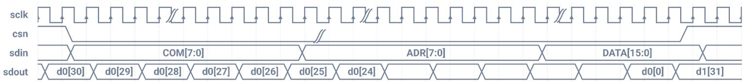
SPI timing takes 32 sclk cycles to enter the 32-bit SPI words into the input shift register of the SPI when csn is LOW. When csn is HIGH, it takes an additional 16 sclk cycles for the SPI controller to decode the SPI commands and read or write to the SPI registers. Including this idle time, an SPI operation will take 48 sclk cycles to complete. It is suggested to generate sclk from clk with a clock division ratio of 4.
