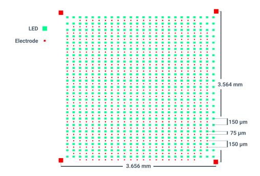
The probe consists of two pieces: an FR4 PCB containing control and power electronics; and a microfabricated glass substrate housing the stimulation and recording ASICs, as well as the active area. A glass well can be affixed to the substrate to create a chamber for cell culture.
